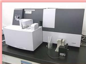
**Laser diffraction Particle size Analyzer**
