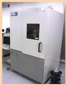
**X-ray diffractometer (XRD)**
