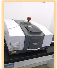
**Fourier transform infrared spectrophotometer (FT-IR)**
