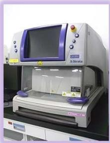
**Energy dispersive X-ray fluorescence measuring instrument (XRF)**
